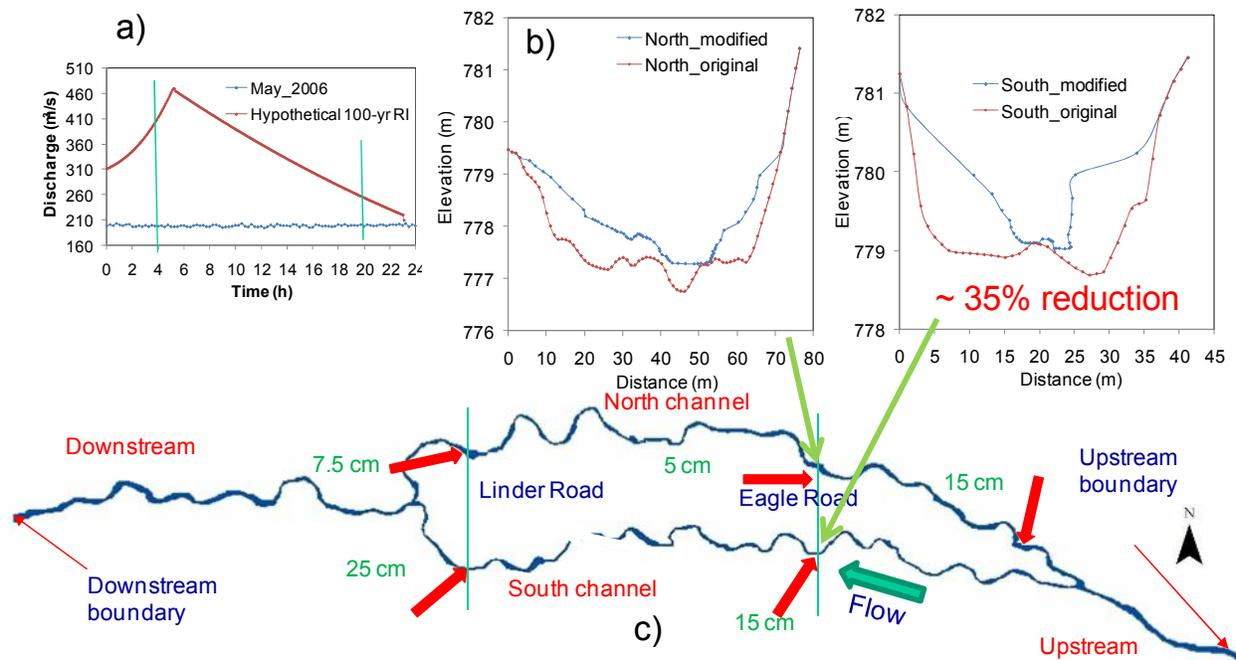
Figure 3: a) hydrographs used in the simulation, b) change and cross-sectional area at the bridges on Eagle Road and c) location of the bridges where measured and simulated Water Surface Elevations (WSEs) were compared and cross-sections are modified. The numerical value (e.g., 15 cm or 6 inches) indicated differences between measured and simulated WSE at that location
