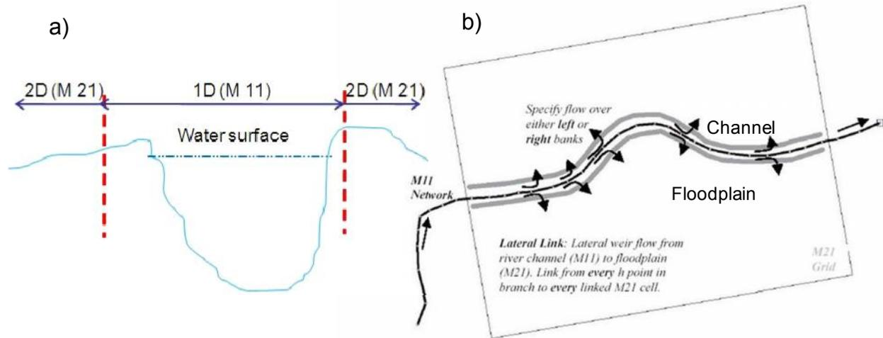
Figure 2: Schematic showing the link between MIKE11 and MIKE21 models using MIKEFLOOD model in a) cross-section and in b) plan views
